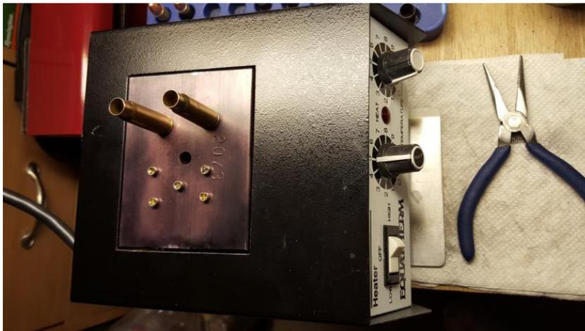
This particular unit was picked up on eBay for \$19.99 + shipping. The test tube holder block is flipped upside down so that the flat bottom can be used to set the primers on for drying. The 2 cases on the block are berdan primed cases that are drying after pressing in moist berdan primers. It also works great to dry reprimed rimfire cases.
